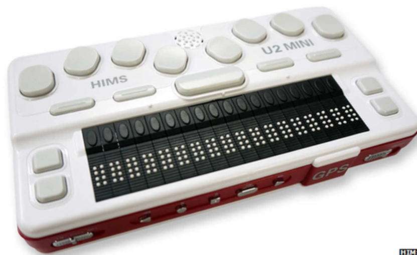
This portable refreshable-screen Braille reader was manufactured as a functional prototype (supports Excel, Twitter, YouTube, and Dropbox); however, its cost exceeds $4,000
